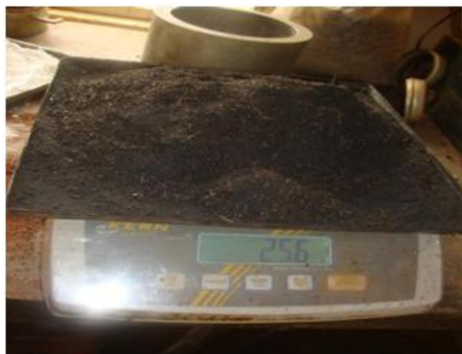
Figure 1: Sample; Bagasse ash on weighing balance
