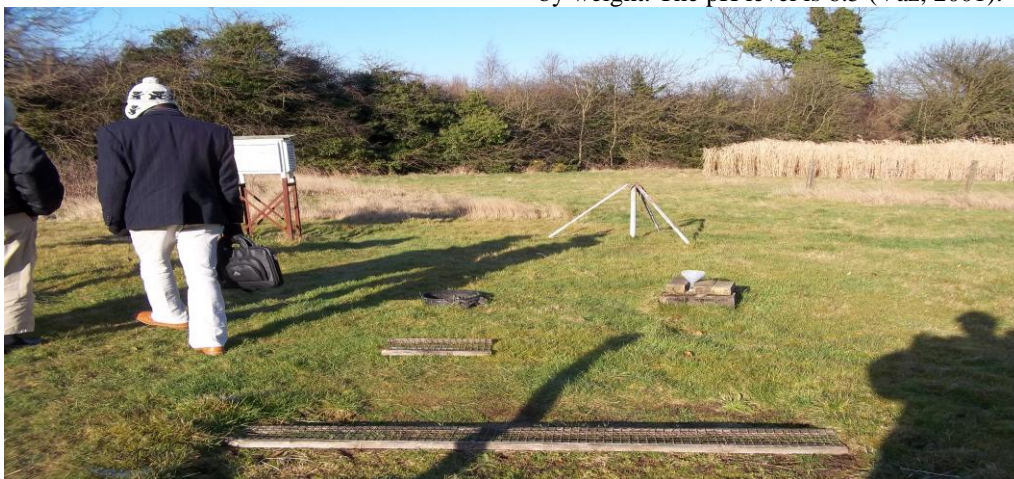
Figure 1: Rain gauge, 60 cm thermometer, slab minimum thermometer, short grass and Miscanthus (elephant) plant at the extreme side of the study area.
