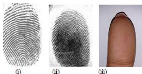
Figure 4: Images of fingerprint by (i) capacitive sensor, (ii) optical sensor, (iii) Digital camera
