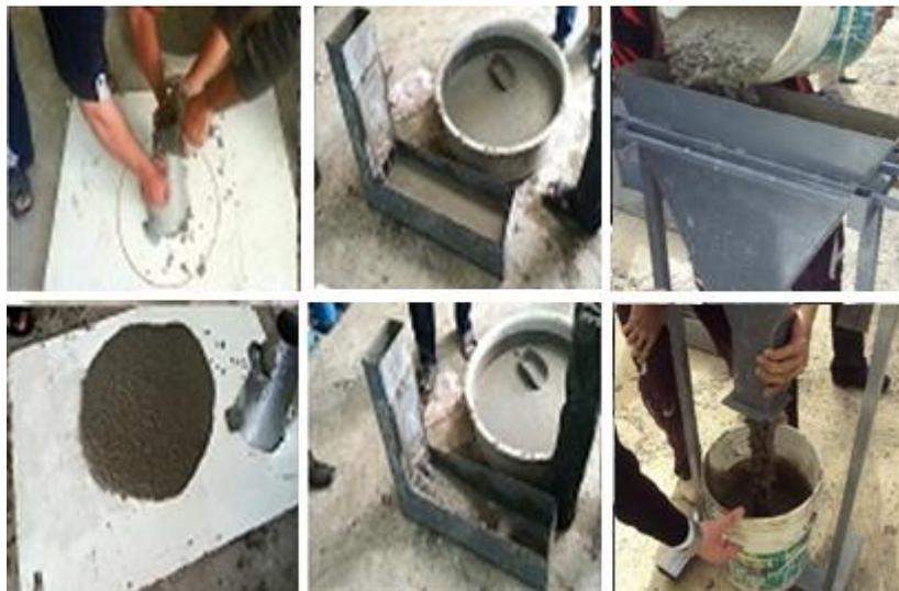
**Plate 1:** Rheological parameters of the SCC
