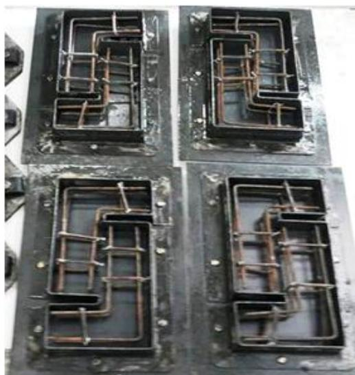
**Plate 2: Steel form with reinforcement**
