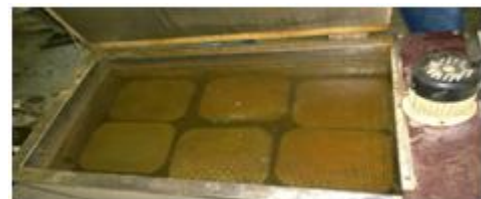
Figure 6: Accelerated Curing of Cubes in Boiler at 60°C
