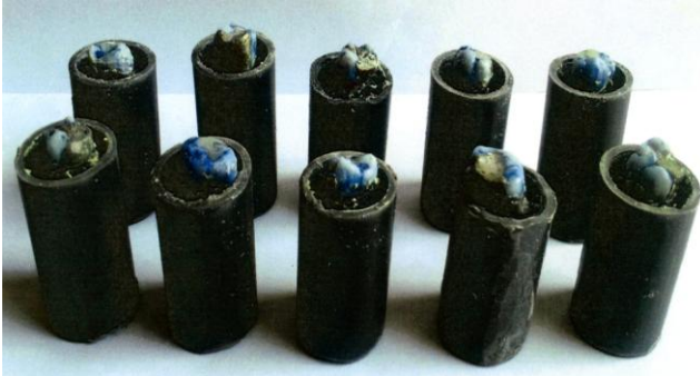
Figure 2: Specimens in groups ready for loading and for the fracture resistant tests
