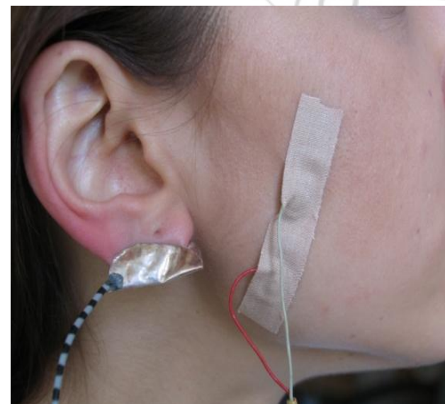
Figure 1: Location of the surface electrode over the belly of examined muscles: anterior temporal muscle (left) and masseter muscle (right).
