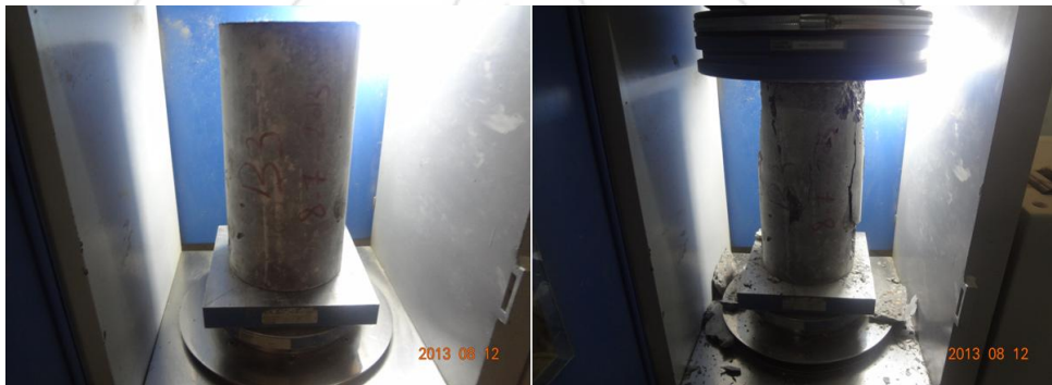
Figure 3.2: Compression strength test cylinder specimens
