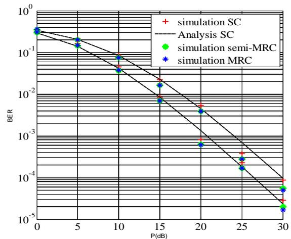
**Figure 6:** Theoretical and simulation BER of the D-AF system with semi-MRC, MRC and SC methods using DBPSK (lower) and DQPSK (upper)
