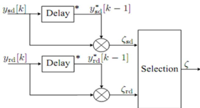
**Figure 2:** Block Diagram of SC at the destination
