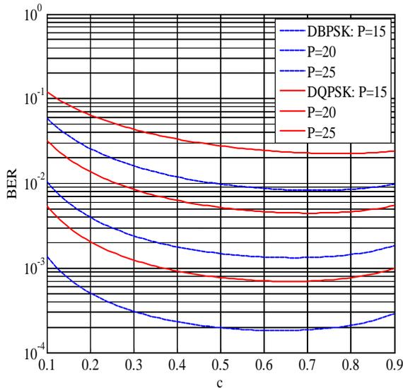
**Figure 3:** BER as a function of power allocation factor  $c$  for  $P = 15, 20, 25$  dB.
