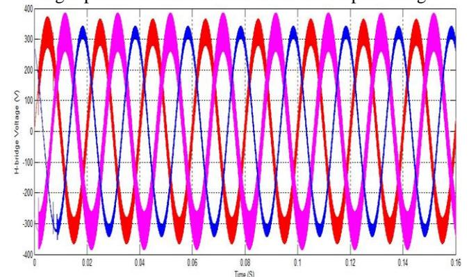
**Figure 8: Single Delta Bridge Cell Voltage Waveform**
