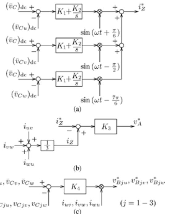
**Figure 3:** Block Diagram of (A) Cluster Balancing Control (B) Circulating Current Control (C) Individual Balancing Control
