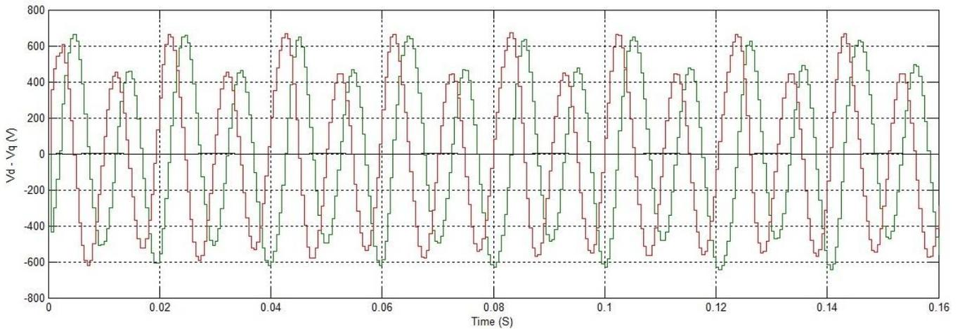
**Figure 10: D – Q Transformation(X – AXIS 1 DIV = 0.02 S; Y – AXIS 1 DIV = 200V)**
