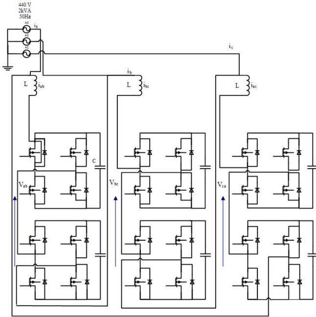
**Figure 2:** Cascaded H-Bridge Inverter
