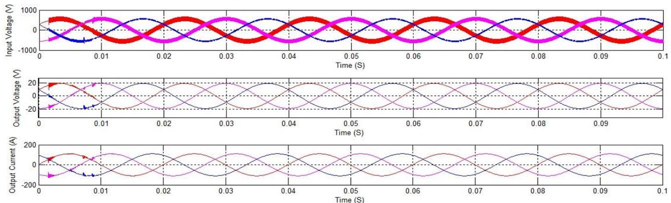
**Figure 12: Output Voltage And Current Waveforms Of The Welding Machine Model (X – AXIS 1 DIV = 0.01 S; Y – AXIS = 20 V; Y – 200 A)**
