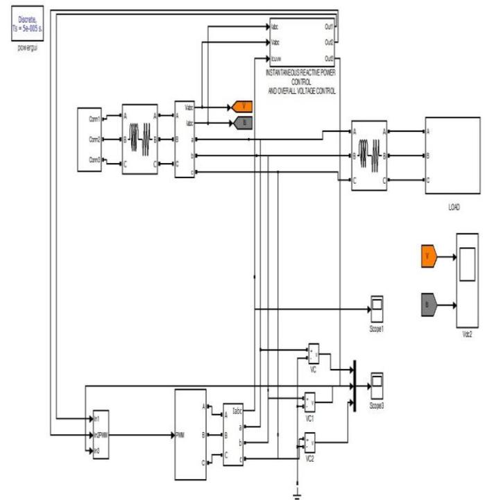
**Figure 5:** Simulink Model of the Proposed SDBC Based STATCOM
