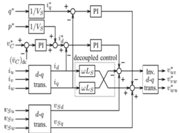
**Figure 4:** Instantaneous Active and Reactive Power Controls and Overall Voltage Control
