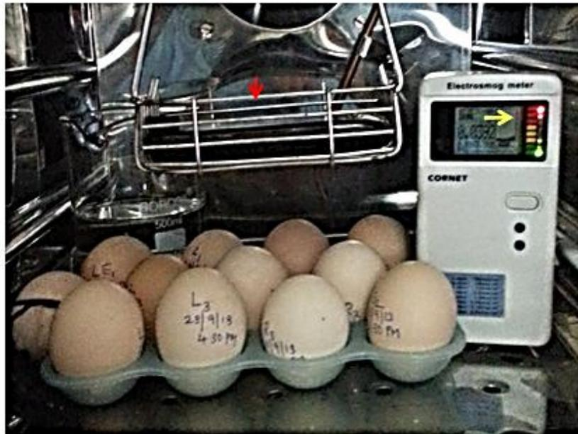
**Fig:1** A Photograph showing the experimental set up. The Mobile phone (red arrow) is hung with a distance of 5cms separating it from the fertilized chicken eggs. A RF meter is kept inside the incubator to check the intensity of radiation (yellow arrow).
