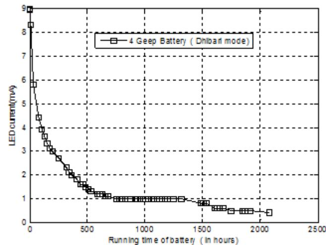
**Figure 7(b):** LED Lamp in low mode of illumination for Geep Battery
