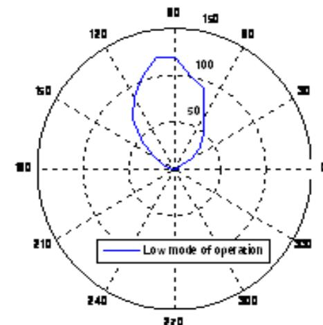
**Figure 6: Radiation pattern of output light intensity of LED lamp**
