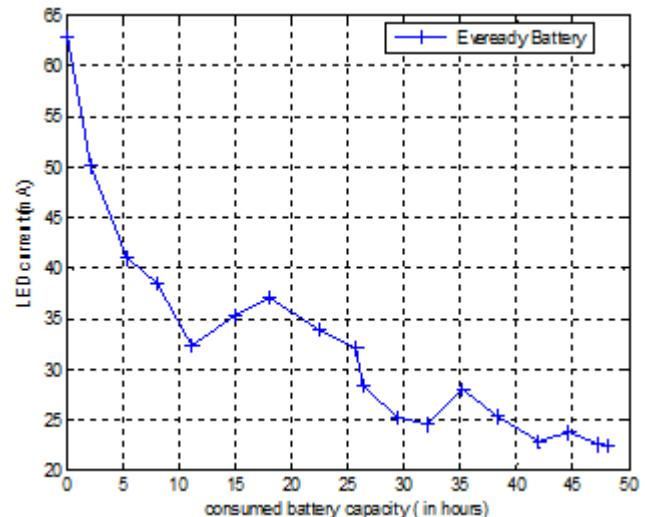
**Figure 7 (c):** LED Lamp in high mode of illumination for Geep and Eveready battery
