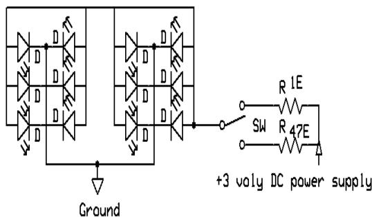
**Figure 4(b): Circuit diagram of LED lamp**
