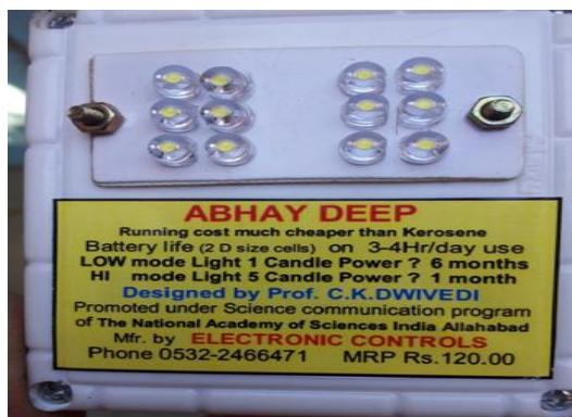
**Figure 4(a): LED Lamp Module**
