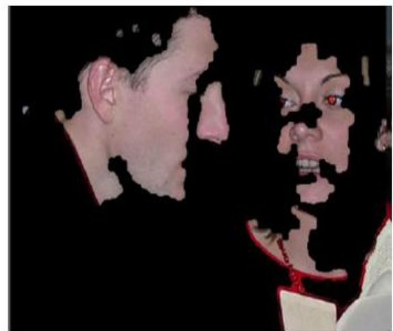
Figure 4(b): Output Image after SVM classification and morphological operation. Figure 4(a) shows the input image and figure 4(b) is the output image after SVM classification and morphological operation.
