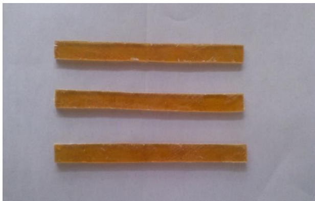
Figure 2: Specimens for bending test
