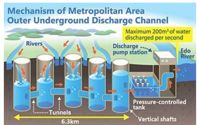
Figure 12: A schematic of the MAOUDC that drains flood water below ground, stores it and eventually discharges it into rivers
