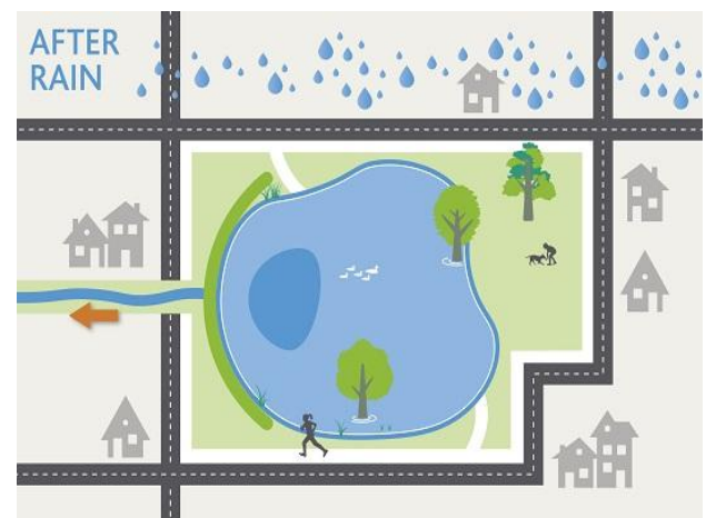
Figure 9: Schematic Explanation of Retarding Basins – After Rain (Source: Melbourne Water)
