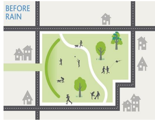
Figure 8: Schematic Explanation of Retarding Basins – Before Rain (Source: Melbourne Water)
