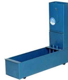
Figure 2: L Box Apparatus
