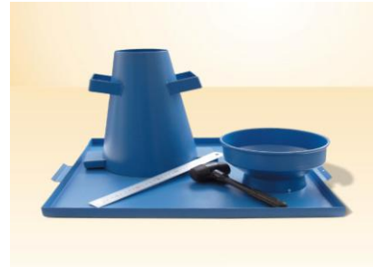
Figure1: Slump flow Test Apparatus
