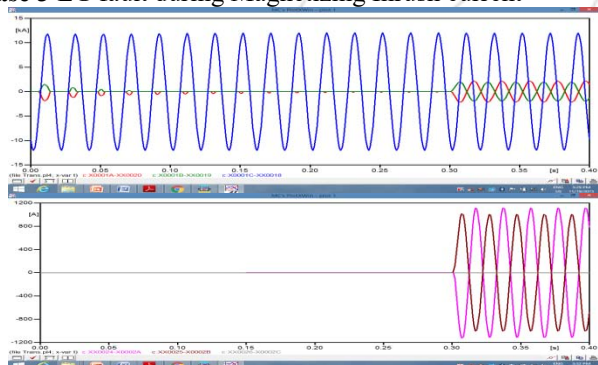
Figure 9: Input and Output Current waveform for LG fault during inrush current
