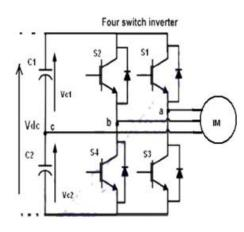
The PWM signal is applied to the switches to obtain the desired switching pattern and hence the desired output. To make this possible we employ the space vector pulse width modulation.
