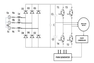
Vector control strategy is widely used in the implementation of four switch three phase inverter. In the six switch topology the active vectors present were six which is now carefully cut down to four in the proposed topology.
