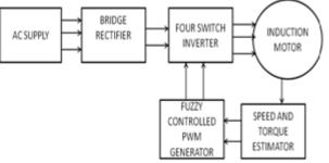
The proposed inverter is used to control the induction motor. Block diagram includes input from power supply, PIC drive
