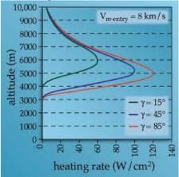
According to above graph, we require ablative materials which can withstand at high peak values.
