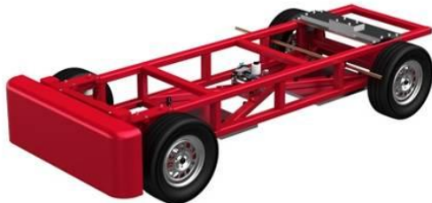
Figure 2.1: Frame Structure of a Fore Wheel Drive
