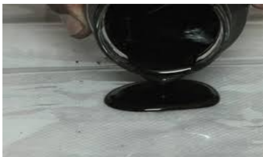
Figure 1.1: Ferrofluid obtained after mixing laser jet tonner and vegetable oil
