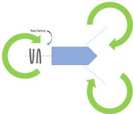
Figure 3: Servo on rear motor for yaw control
