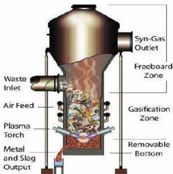
Figure 1: A Plasma Gasifier
