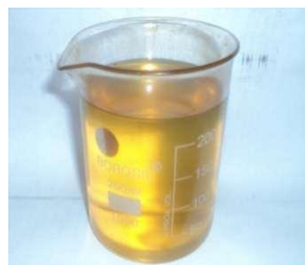
Figure 1: Pure Transformer Oil
