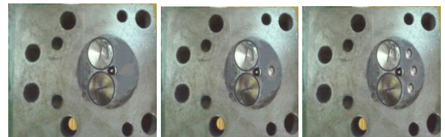
Figure 2: Conventional cylinder head and Cylinder head with oval shape dimples
