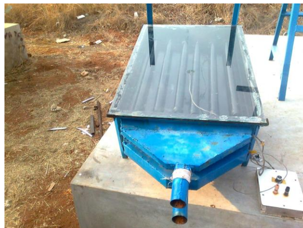
Figure 5: Image of Fabricated and Assembled Solar Air Heater
