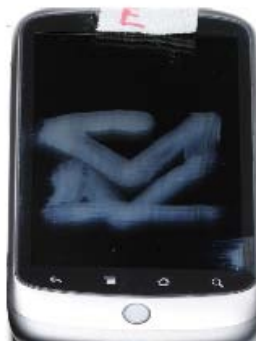
Figure 2: the smudging effects that enable an attacker to launch a smudge attack
