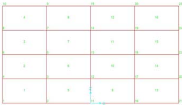
Figure 3: Discretization of the thin plate (rectangular finite elements)
