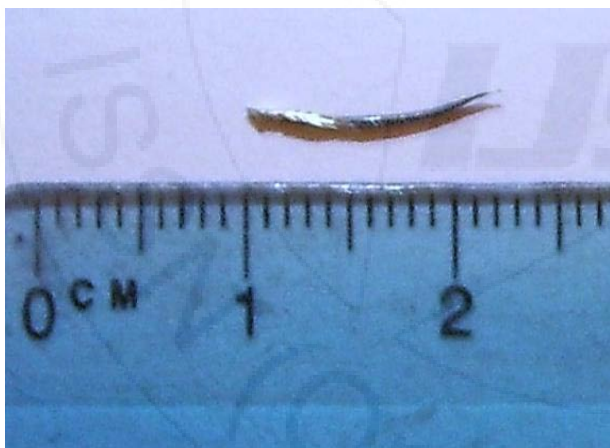
Figure 4: The extracted silver point observation revealed significantly corroded apical portion. In the coronal part the core is shiny due to mechanical removal of the superficial layer by the ultrasound tip.
