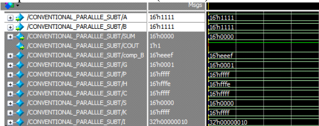
Figure 8: Functional simulation waveform
