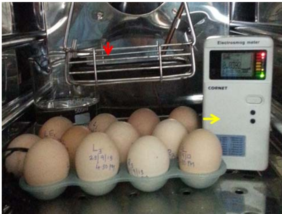
Figure 1: A Photograph showing the experimental set up. The Mobile phone (red arrow) is hung with a distance of 5cms separating it from the fertilized chicken eggs. A RF meter is kept inside the incubator to check the intensity of radiation (yellow arrow).
