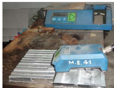
Figure 5: Set up for HOMMEL surface roughness tester
