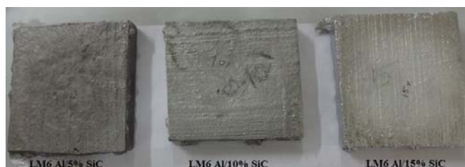
Figure 2: Casted composite materials after stir casting
