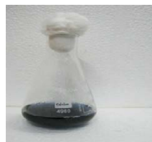
Figure 5: Calcium presents with EDTA with metallic blue end point.
