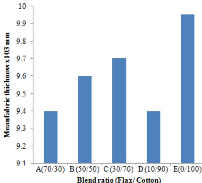
Figure 3: Fabric Thickness versus Blend ratios
