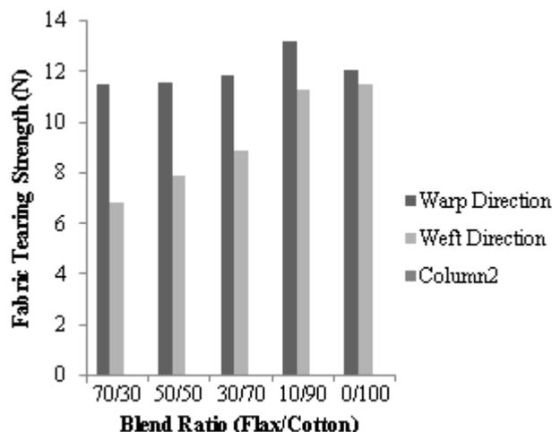
Figure 7: Fabric Tearing Strength Versus Blend ratio
