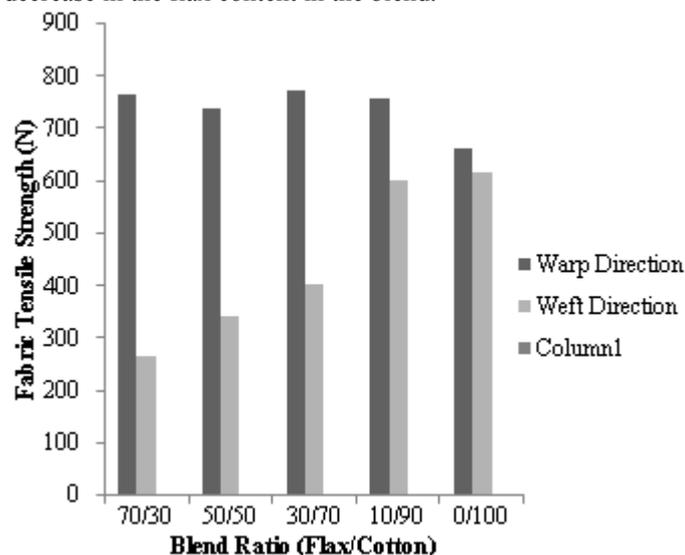
Figure 8: Fabric Tensile Strength versus Blend ratio
