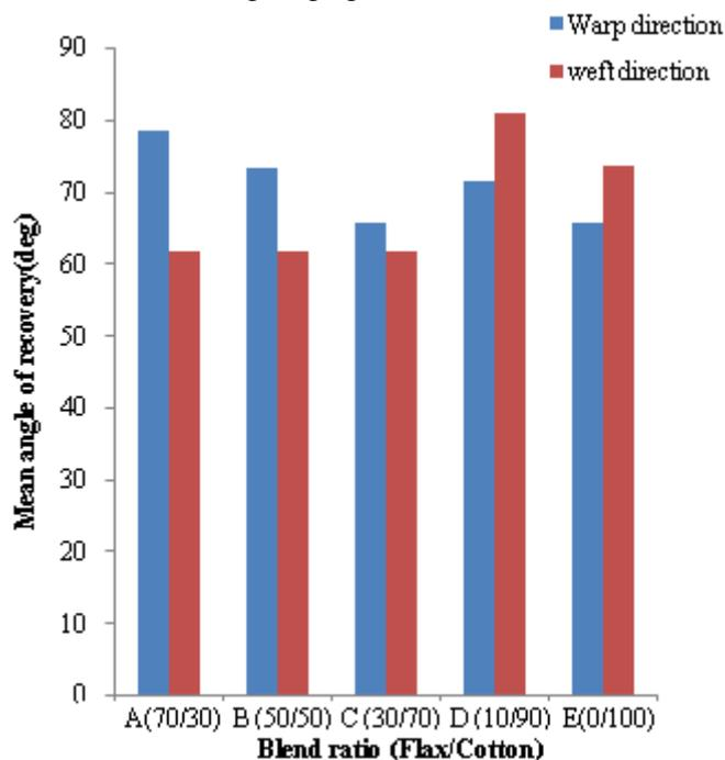
Figure 5: Fabric Angle of Recovery versus Blend ratio
