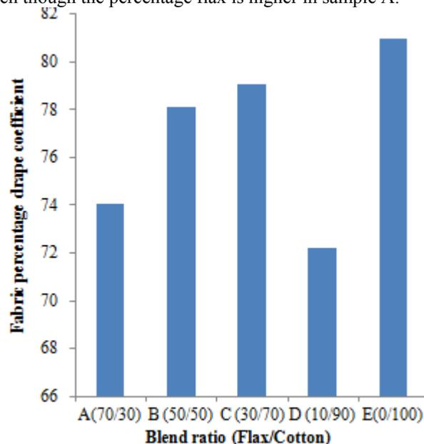
Figure 4: Fabric Percentage drape coefficient versus blend ratio
