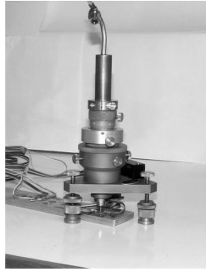
Figure 2: Hole drilling apparatus [17]
