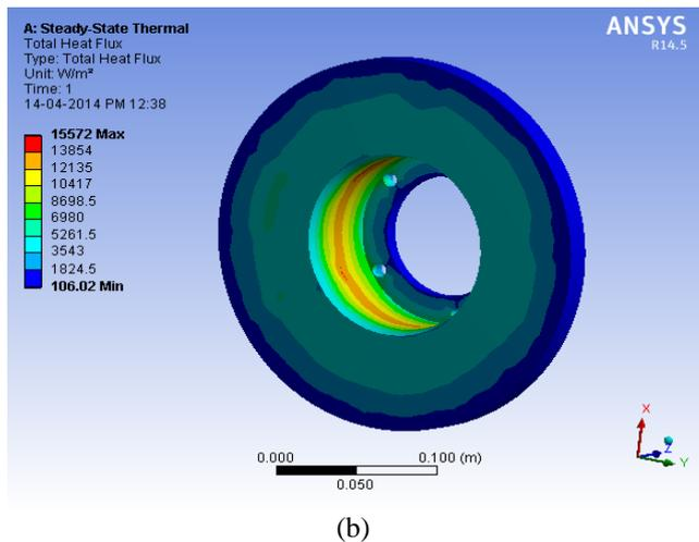
Figure 6.2: (a) & (b) Solid disc brake S-2 Glass Fiber
