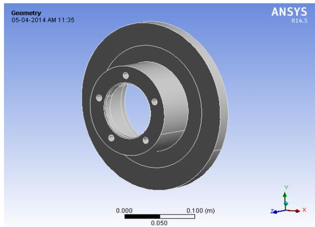
Figure 5.7: (a) Solid type disc brake imported in ANSYS
