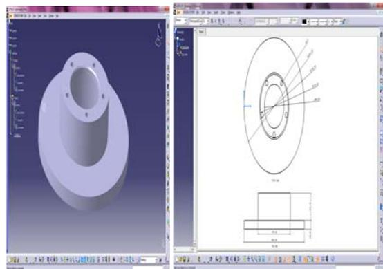
Figure 3.1: Solid model of Solid disc brake & Drafting
