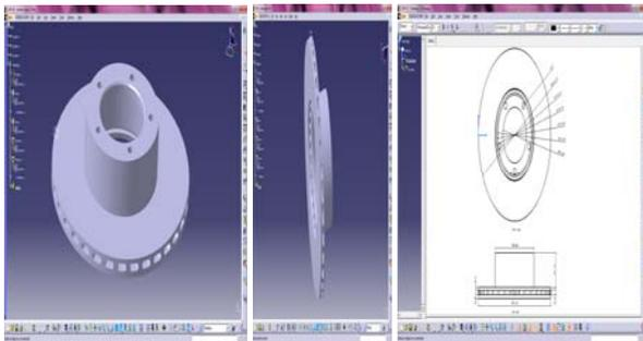
Figure 3.2: (a) and (b) Solid model of Ventilated disc brake and Drafting of Ventilated disc brake
