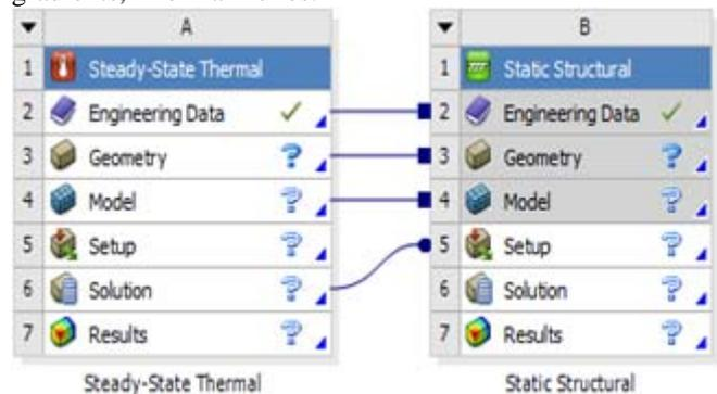
Figure 5.4: Thermal-Structural Coupling (Ref) in ANSYS Workbench
