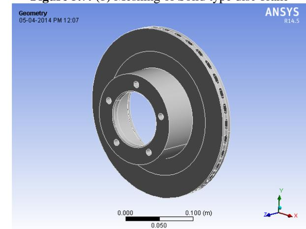
Figure 5.8: (a) Ventilated type disc brake imported in ANSYS
