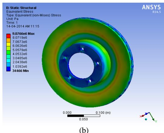
Figure 6.3: (a) & (b) Ventilated disc brake S-2 Glass Fiber
