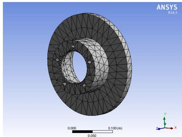
Figure 5.7: (b) Meshing of Solid type disc brake
