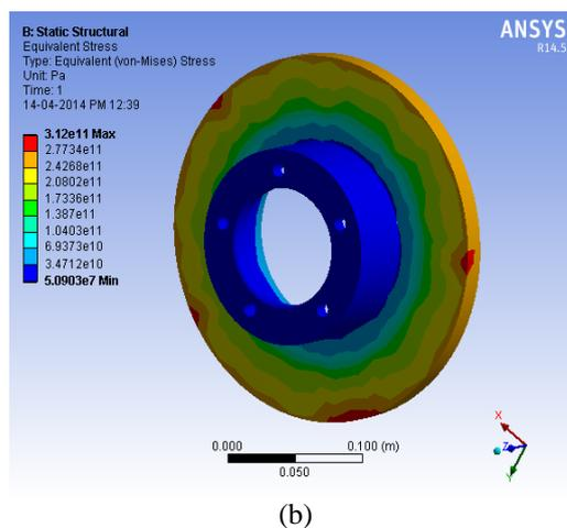
Figure 6.4: (a)&(b) Ventilated disc brake S-2 Glass Fiber
