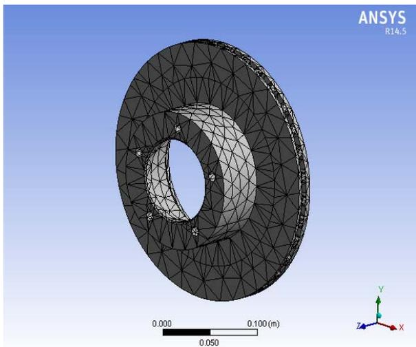
Figure 5.8: (b) Meshing of Ventilated type disc brake
