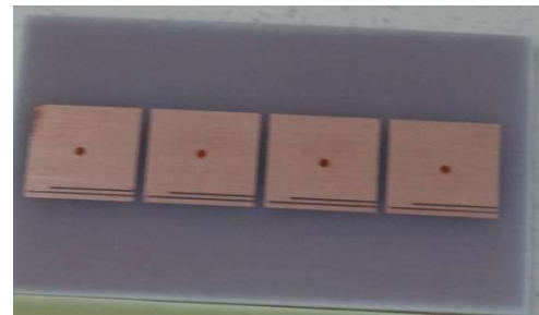
Figure 12: Fabricated structure of Mushroom-like EBG structure with two slit-tops
