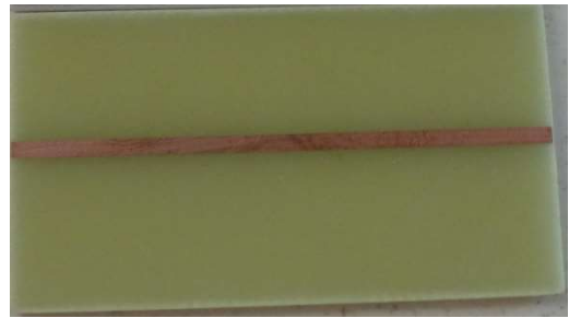
Figure 10: Fabricated structure of Microstrip line
