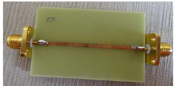
Figure 13: Fabricated structure of Mushroom-like EBG structure with two SMA connectors on both side
