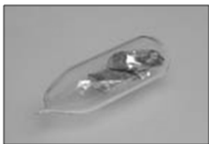
Figure 8: Ingot of compound semiconductor material
