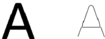
Figure 3: Input image Skeletonization Image
