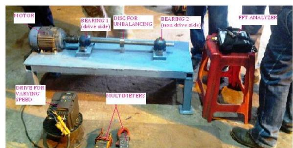
Figure 2.1: Experimental Setup for Deep Groove Ball Bearing Test
