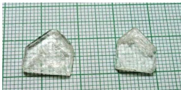
Figure 1: Photograph of as grown BaTr crystal
