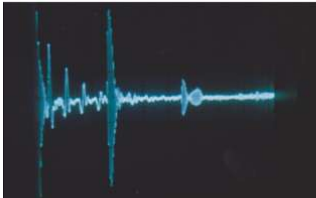
Figure 2: Transmitted pulse of Ultrasonic wave
