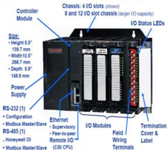
Figure 1: HC900 Controller with details
