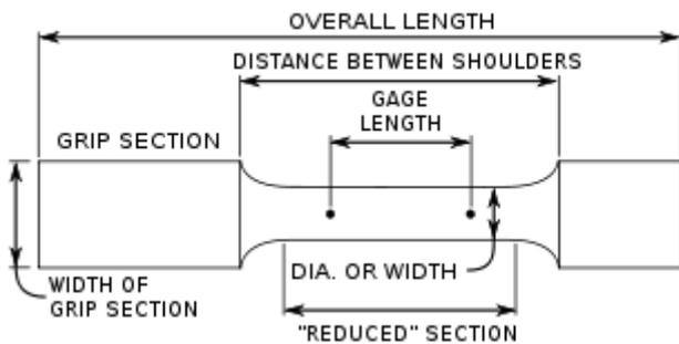
Figure 6: Tensile Specimen
