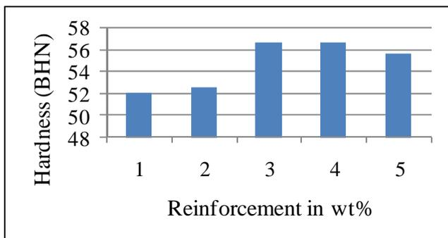
**Figure 16:** Hardness value for different wt% reinforcement
