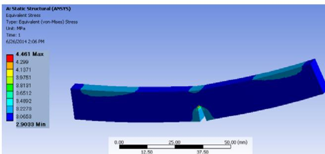
Figure 12: Stress distribution from finite element simulations
