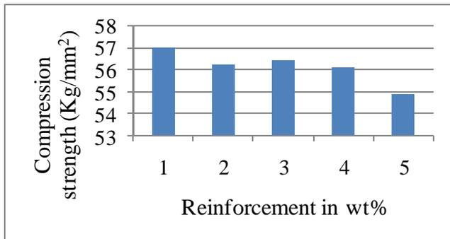
**Figure 15:** Compression strength for different wt% reinforcement
