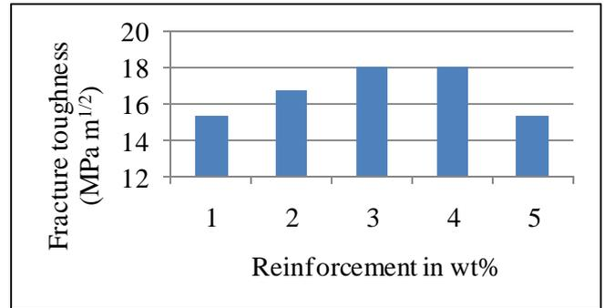
Figure 13: Variation of Fracture toughness with different Wt% reinforcement
