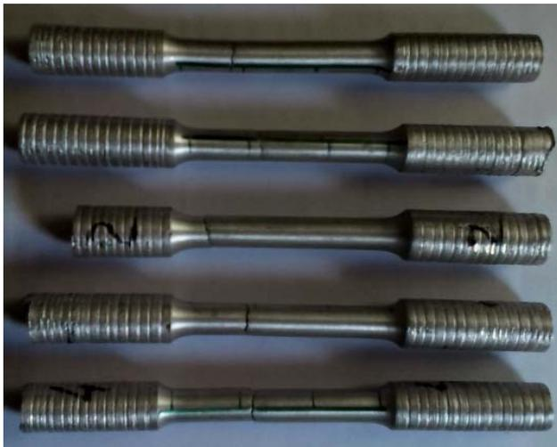
Figure 7: Specimens for Tensile test
