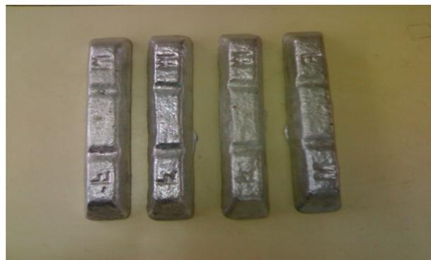
Figure 1: Ingot Structure of Al 356
