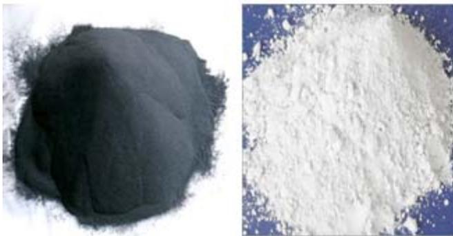
**Figure 2:** Zirconium Silicate **Fig 3:** Silicon carbide
