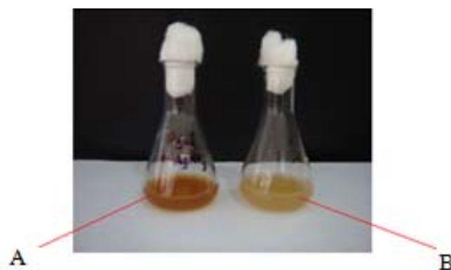
A) Penicillium chrysogenum treated with \text{AgNO}_3 B) Penicillium chrysogenum after sonication (without \text{AgNO}_3 ) Figure 1: Intracellular biosynthesis of silver nanoparticles by using fungi Penicillium chrysogenum
