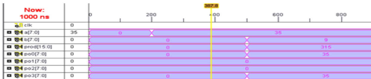
Figure 7: Output waveform of shift and add multiplier
