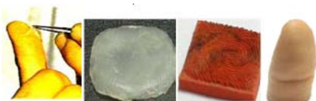
Figure 2: Shows Fake Fingerprint using Rubber, Silicon,
