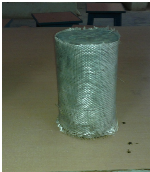
Figure 4: Woven GFRP sheet installed on cylinder specimen
