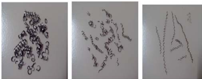
Figure 6: Chips formed during random trials
