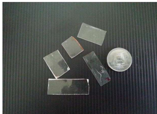
Figure 3: Photographs of the samples of PMMA and Wax prepared for using as substrates for the SRR
